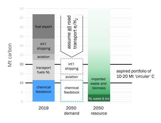
**Figure 6**: The current situation and the outlook for the challenge area of oil products and chemical feedstock. The 2019 product slate is almost entirely oil-based and corresponds to ca. 1 million barrels per day of oil. The 2050 demand outlook is based on assumptions discussed in the text. The 2050 resource outlook illustrates that domestic resources of circular carbon (biomass and waste) fall very much short of resourcing what could be the level for an aspired portfolio: 10-20 MtonC.
